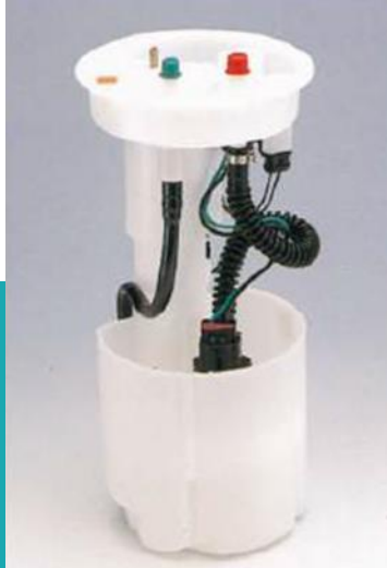
Fuel pump unit
