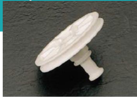
Brake booster piston relay
